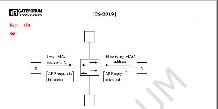
ARP is a network protocol used to find the Hardware (MAC) address of a host from an IP address. It is a request reply protocol.
