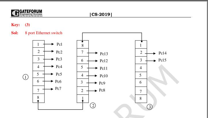
:. To connect 15 machines in a LAN using 8-port Ethernet switches, we require 3 switches.
